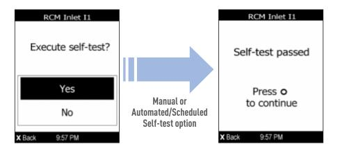
Raritan RCM self-test function turns on a test AC current with an extra wire that runs through the sensor. The circuitry is working properly if it can sense a difference when the test current source is turned on.
