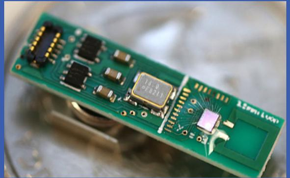
The Bluetooth transmitter chip is connected to a magnetic monopole antenna, which acts as an integral part of the transmitter's resonator circuit. The left half of the circuit board is only for test purposes. This device consumes 0.6mW at full power transmission and is half the size of a dime.
