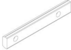
1 x Pin Bracket (250-80-0009-00) Dimensions (WxHxD): 43.6mm x 6.6mm x 3.2mm
