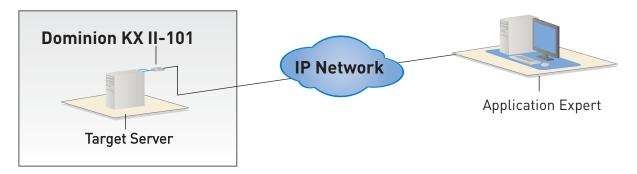
If an outside expert is needed to solve a problem, the technician can connect the KX II-101 to the network for secure KVM-over-IP access.
