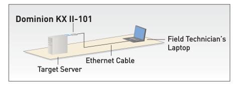
As a "mobile crash cart", the KX II-101 can be plugged into the target server and the technician's laptop for easy access.
