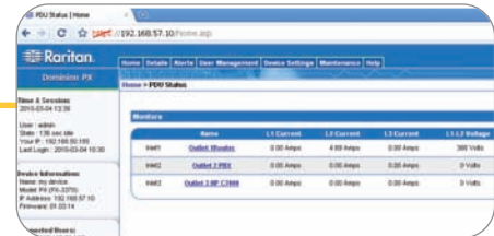
Remote power monitoring, including current (amps), voltage, power (kVA, kW) and energy consumption (kWh)
