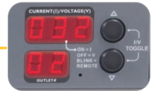
At-the-rack power monitoring of current (amps), voltage and active power (watts)
