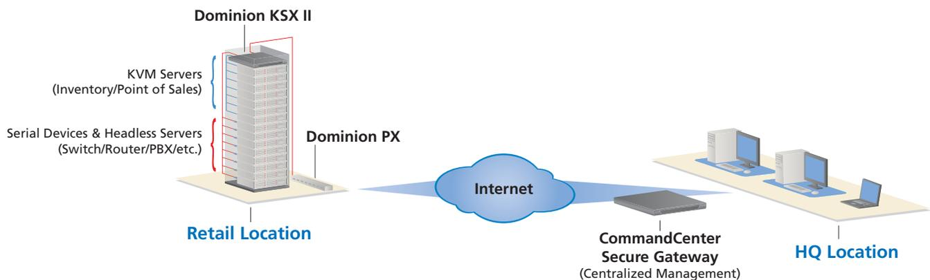
In this example, the retail locations are using the Dominion KSX II for remote out-of-band access and control of all of their IT devices. They are also using the Dominion PX, an intelligent PDU for emergency reboots and power monitoring. This, combined with the centralized management tool, CommandCenter Secure Gateway, provides an optimal way for an HQ-based IT team to remotely troubleshoot and maintain their equipment and maximize uptime.
